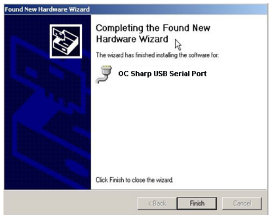
Fig. 3-7: Driver installation completed
