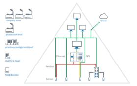
The SIG200 enables two parallel communication channels: One With IO-Link technology and the Sensor Integration Gateways for edge computing for the PLC and one for cloud computing for Industry 4.0 applications. That's what we call "Dual Talk".
