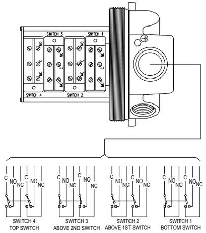
**Figure 4:** Wiring for switch type D. 1, 2, or 4 switches.
