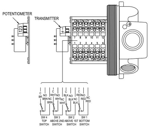
**Figure 8:** Wiring for switch types B, C, I, R, V, and W. 1, 2, 4, or 6 switches. Switch types B and I have "+" and "-" terminals.
