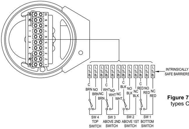
**Figure 7:** Intrinsically Safe wiring for switch types C, R, V, and W. 1, 2, or 4 switches
