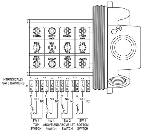
**Figure 2:** Intrinsically safe wiring for switch types A, G, H, M and T. 1, 2, or 4 switches
