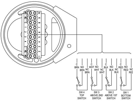
**Figure 6:** Wiring for switch types C, R, V and W. 1, 2, or 4 switches.
