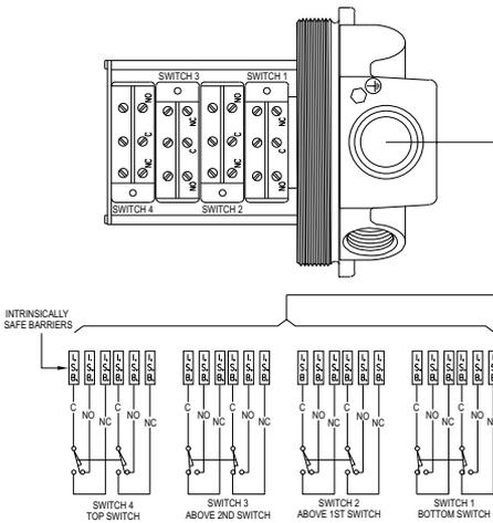
**Figure 5:** Intrinsically Safe wiring for switch type D. 1, 2, or 4 switches.
