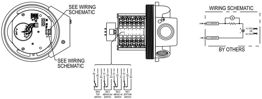
**Figure 12:** Intrinsically Safe wiring for transmitter with HART® communication output. Refer to proper switch figure if unit has switches as well.
