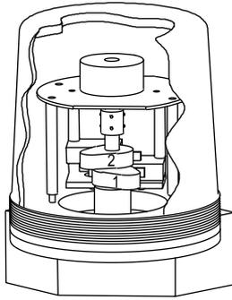
Models 19XXX, 39XXX and 49XXX Rotary Position Indicating Switches contain a 4-20 mA transmitter with HART® communication and two Single Pole Double Throw (SPDT) switches. Models 190XX, 390XX and 490XX contain a 4-20 mA transmitter with HART® communication only, no switches.
