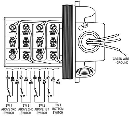
**Figure 3:** Wiring for factory sealed leads option. 1, 2, or 4 switches. Switch 1 wires are red, switch 2 wires are black, switch 3 wires are white, and switch 4 wires are brown. Wires are labeled C, NO, NC.
