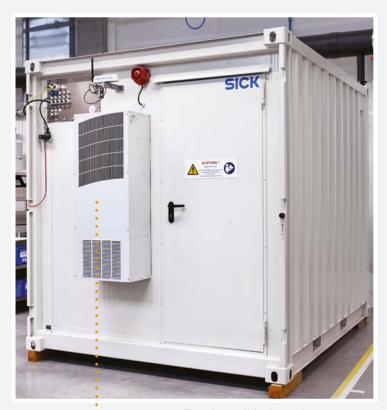
The air conditioning unit ensures consistent ambient conditions, thus further increasing the reliability of the measurement.
