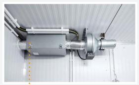
The **pipe fan** with large filter cassette ensures good ventilation, even in very dusty environments. The integrated differential pressure measurement signals when it is time to clean the filter.
