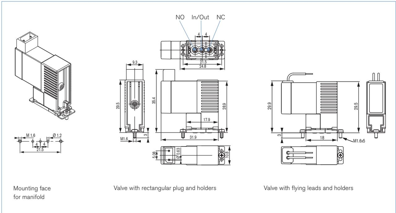
Valve dimensions [mm] with tube spigots sideways and UNF 1/4 -28
