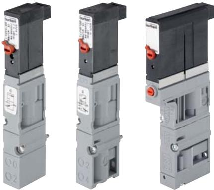
The solenoid valve Types 6524 and 6525 consist of a 6144 flipper pilot valve and a pneumatic seat valve. The principle allows switching of high pressures together with low power consumption and fast response times. The pilot valves are equipped with manual override as a standard.
