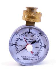
Marsh Instruments Water Test Gauge is designed to connect directly to a standard 3/4" water faucet or hose. The max pointer included on the Water Test Gauge allows you to monitor a peak operating or surge pressure point.
