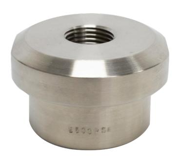
The Model 13040 All Welded Seal is designed for up to to 4 1/2" bourdon tube gauges with pressure ranges from vacuum to 1000 psi. Available in all 316 Stainless Steel or Hastelloy C process housing and diaphragm, with threaded connections. Optional flushing connections also available.
