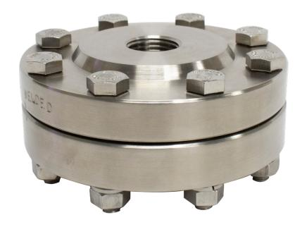
The Model 14040 Welded Diaphragm Seal is a welded diaphragm-to-upper design allowing the upper housing to be removed with the instrument in place without losing fill. Available in threaded connections for pressures from vacuum to 2,500 psi. Fill/bleed port screw in the upper is standard and an optional flush connection is available.
