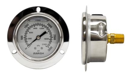
Marsh Instruments Severe Service Liquid Filled Gauges are designed to perform in rugged and harsh environmental conditions, especially where pulsation or vibration is a problem. Liquid Filled Gauges offer a significant cushioning and dampening effect, reducing pointer flutter and lubricating the internals.
