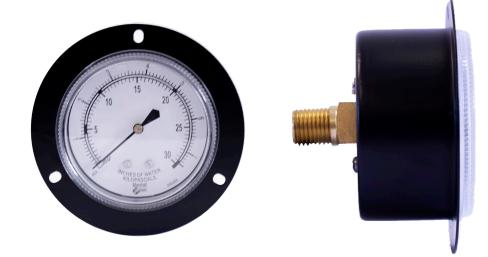
Low Pressure Gauges from Marsh Instruments incorporate a diaphragm element allowing for accurate low-pressure readings in support of a variety of applications, with ASME Grade A 2/1/2% accuracy for ranges above 30" of water. Available ranges include vacuum and pressure in inches of water, ounces per square inch, kilopascals, and millimeters of mercury.
