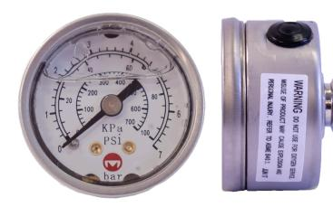
Marsh Instruments Severe Service Liquid Filled Gauges are designed to perform in rugged and harsh environmental conditions, especially where pulsation or vibration is present. Liquid Filled Gauges offer a significant cushioning and dampening effect, reducing pointer flutter and lubricating the internals.
