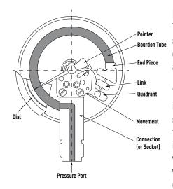
Bourdon tube pressure gauges are widely usedin all branches of industry. The construction is simple yet rugged, and operation does not require any additional power source. The Bourdon tube element is directly exposed to the medium being measured and is normal made of copper alloy (brass) or stainless steel as the application demands.
