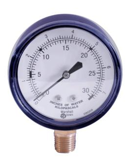
Low Pressure Gauges from Marsh Instruments incorporate a diaphragm element allowing for accurate low-pressure readings in support of a variety of applications, with ASME Grade A 2/1/2% accuracy for ranges above 30" of water. Available ranges include vacuum and pressure in inches of water, ounces per square inch, kilopascals, and millimeters of mercury.
