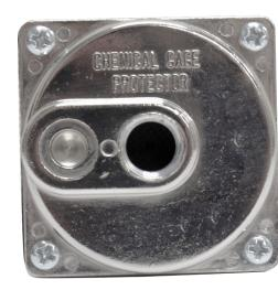
The Model B8498 Gauge Protector is designed for extremely high volume displacement. Ideally suited for gauges and instruments with operating pressures up to 200 psi and vacuum applications. Available in 1/4" threaded connections and chrome plated zinc construction. A 3/8" flush plug is staindard in the process side housing.
