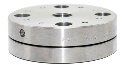
The Model 140FL Welded Diaphragm Seal is a welded diaphragm-to-upper design allowing the upper housing to be removed with the instrument in place without losing fill. Available in threaded connections for pressures from vacuum to 2,500 psi. Fill/ bleed port screw in the upper is standard and a flush ring option is available.
