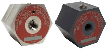
The Model 12000 Serviceable Mini Diaphragm Seal is designed for gauges and instruments with operating pressures of 2500 psi with stainless and 500 psi with PVC models. Ideally suited for small applications and corrosive installations. The optional "Easy Clean Out" feature allows the removal of the process side housing without losing the instrument side fill fluid. Fill/bleed screwport in the instrument side housing, and stainless steel build screws are standard.
