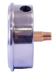
Marsh Instruments Severe Service Liquid Filled Gauges are designed to perform in rugged and harsh environmental conditions, especially where pulsation or vibration is a problem. Liquid Filled Gauges offer a significant cushioning and dampening effect, reducing pointer flutter and lubricating the internals.
