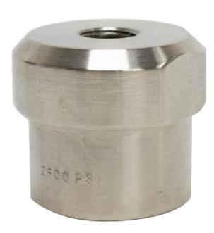
The Model 13000 Mini Welded Seal is designed for up to to 3 ½" bourdon tube gauges with a minimum range of 0-60 psi. The maximum operating pressure is 2,500 psi at 100°F. Available in all 316 Stainless Steel or Hastelloy C process housing and diaphragm.
