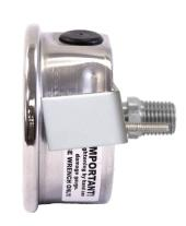
Marsh Instruments Severe Service Liquid Filled Gauges are designed to perform in rugged and harsh environmental conditions, especially where pulsation or vibration is a problem. Liquid Filled Gauges offer a significant cushioning and dampening effect, reducing pointer flutter and lubricating the internals.
