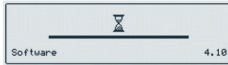
Fig. 23: Initial commissioning. The software version is displayed in the lower right corner.
