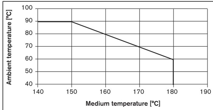
Fig. 1: Combination of medium temperature / ambient temperature
