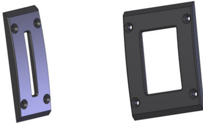
Figure 7: Laser (sender) window to the left, camera (receiver) window to the right
