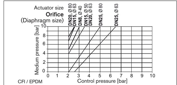
Fig. 9: Control function I, elastomer diaphragm, actuators  $\varnothing$  40 – 80 mm
