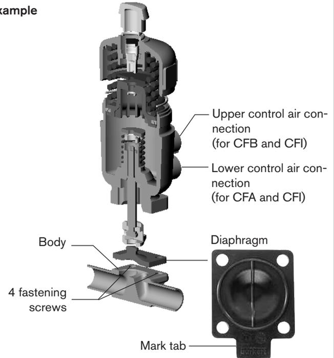
Fig. 32: Replacement of diaphragm
