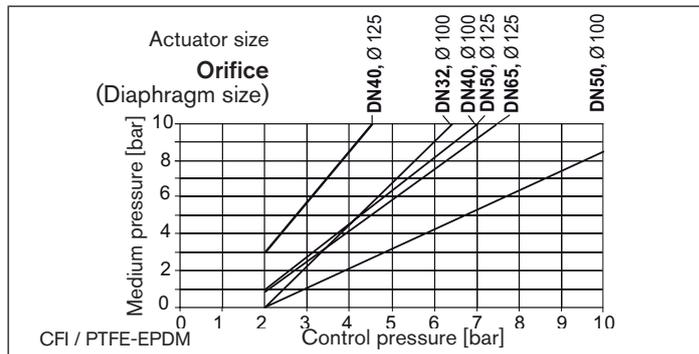
Fig. 12: Control function I, PTFE EPDM diaphragm, actuators  $\varnothing$  100 – 125 mm
