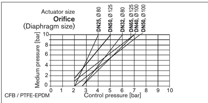
Fig. 16: Control function B, PTFE EPDM diaphragm,
