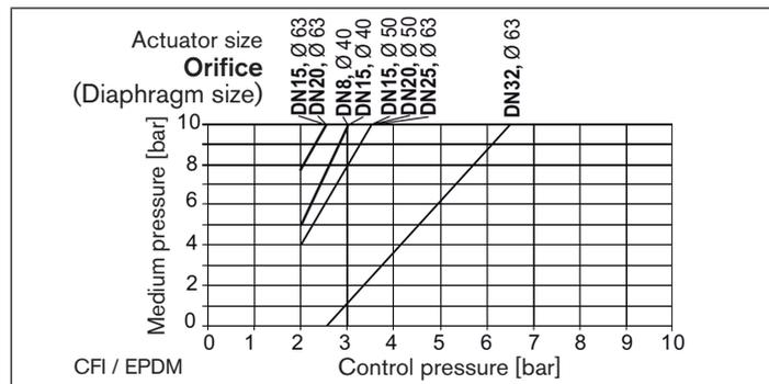
Fig. 17: Control function I, EPDM diaphragm,
