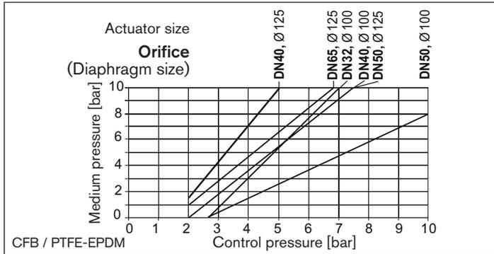
Fig. 8: Control function B, PTFE elastomer diaphragm, actuators  $\varnothing$  100 – 125 m
