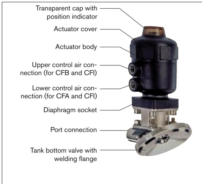
Fig. 23: Structure and description Type 2033
