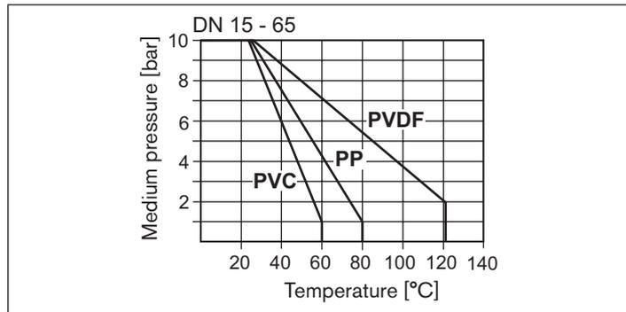
Fig. 4: Graph of medium pressure / Medium temperature
