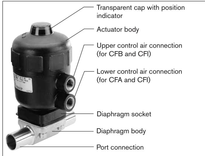
Fig. 21: Structure and description Type 2030, 2031 and 2031 K
