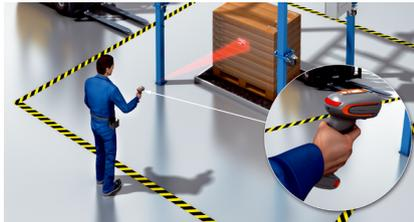
Universal code reading in the field of logistics automation: The large reading distance enables the detection of codes from a wide range of distances.
