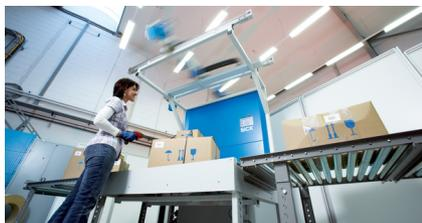
Especially when it comes to stationary track and trace systems, manual mobile code reading is often required as a back-up – this can be done economically with AUX loop-in.
