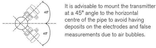
The flow rate transmitter can be installed into either horizontal or vertical pipes. Mount the 8041 transmitter in these correct ways to obtain an accurate flow measurement.
