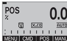
In the AUTOMATIC operating state normal controlled operation is implemented. (The symbol for AUTOMATIC
