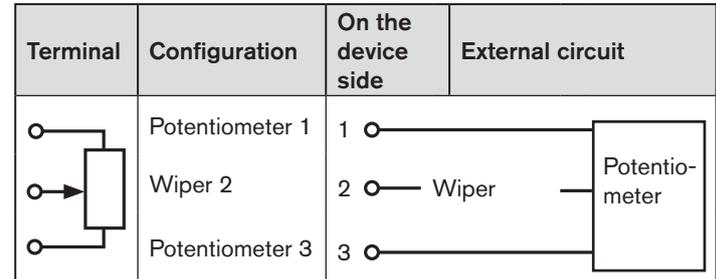
Tab. 16: Terminal assignment; potentiometric position sensor
