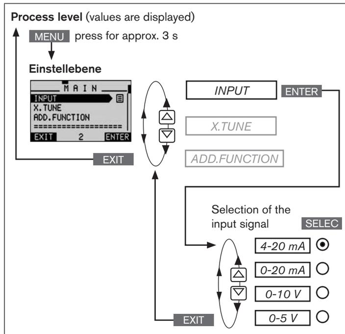
Fig. 24: Operating structure *INPUT*; Input the signal
