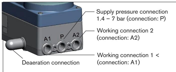
Fig. 15: Pneumatic installation / Location of the connections
