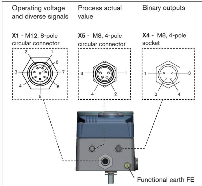
Fig. 19: Designation of the circular connectors and contacts
