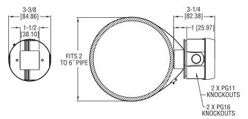
The **SERIES TE-SNW** Surface Temperature Sensors non-intrusively measures the process temperature in hot and cold water loops in buildings. In order to work with most common building controllers, the output of the sensor can be chosen from 6 different RTD and Thermistor curves.
