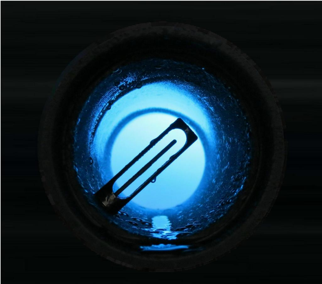
Kurz thermal mass flow meters provide excellent measurement capabilities in dry gas flows. They have proven durability, accuracy, and repeatability. Where all thermal meters have been largely ignored is in the biogas environment. Condensation levels in biogas fluctuate as temperatures change during the day, and it's the highly unreliable readings from those liquid droplets vaporizing on the sensors that make wastewater and landfill operators dismiss thermal meters.
