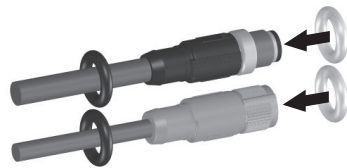
Figure 13: Assembly of IP69K protective housing, with use of the Ethernet connection – Step 1
